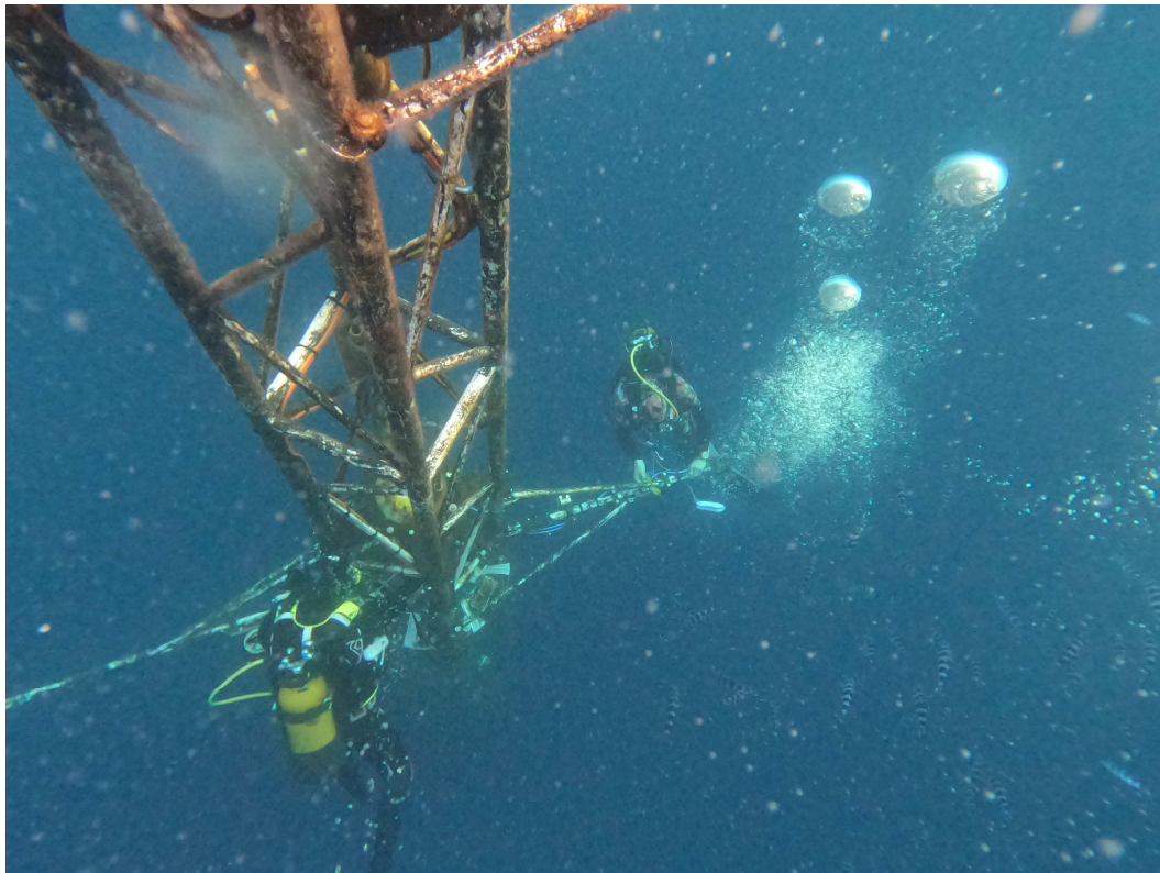
Cleaning of the BOUSSOLE buoy sensors by the divers.
